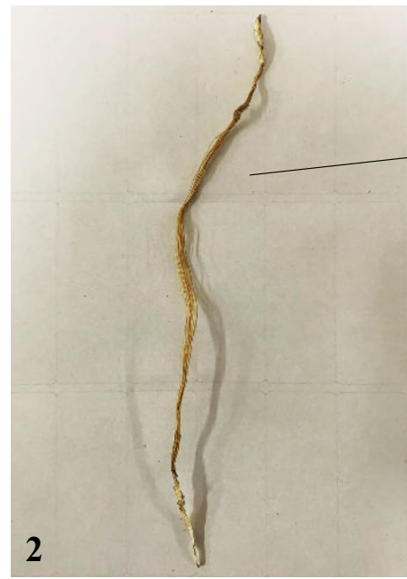
Sisal fiber strand after being extracted from the specimen
