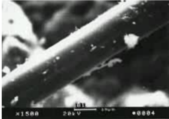
Photo 1 PVA Fibre surface Without microsilica
