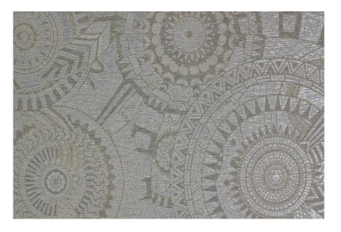
Possibility of ennobling fibre cement by marking abstract and/or geometric designs or replicating wood grain.
