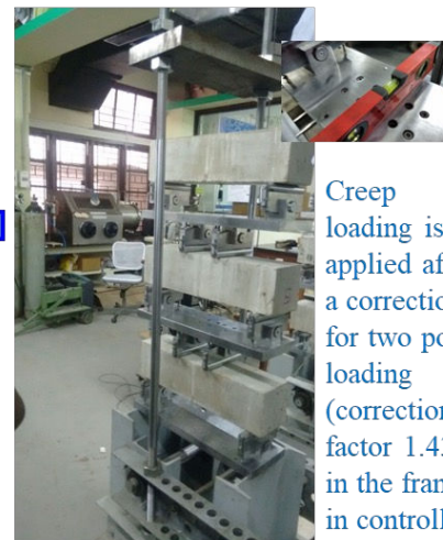
Pre cracking done according to EN 14651 with CMOD control
