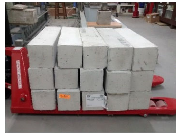
Specimens in controlled environment, Temp 25°C and 65% RH
