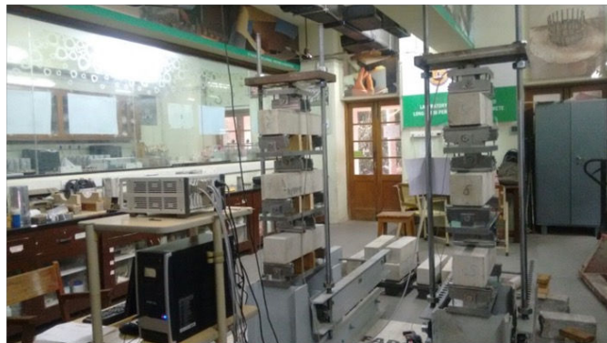
Load cells measure load and CMOD is measured by clip gauges which is connected to DAQ which monitors continuously
