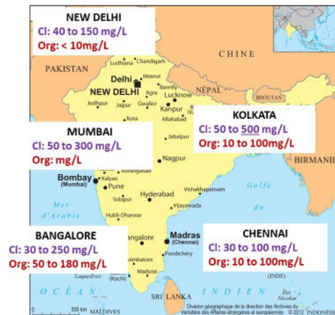
Chloride content of water used for concrete in different regions
